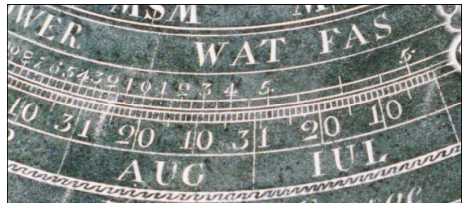
Fig. 8. Part of the EoT scale on the Lacock Abbey dial. Note the division to half-minutes and the day numbers increasing right to left.
