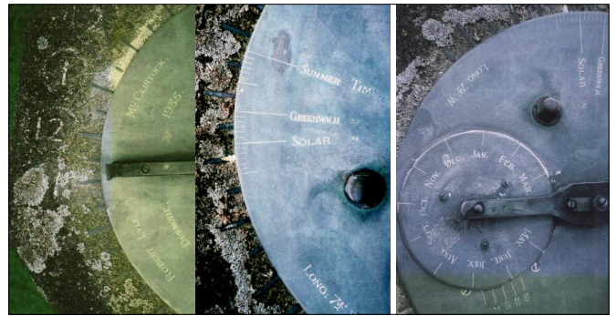
Figs. 3a,b,c. Details of the 1935 heliochronometer showing (left to right): a) the cast hour numerals; b) the vernier scale on the edge and c) the date disk.
