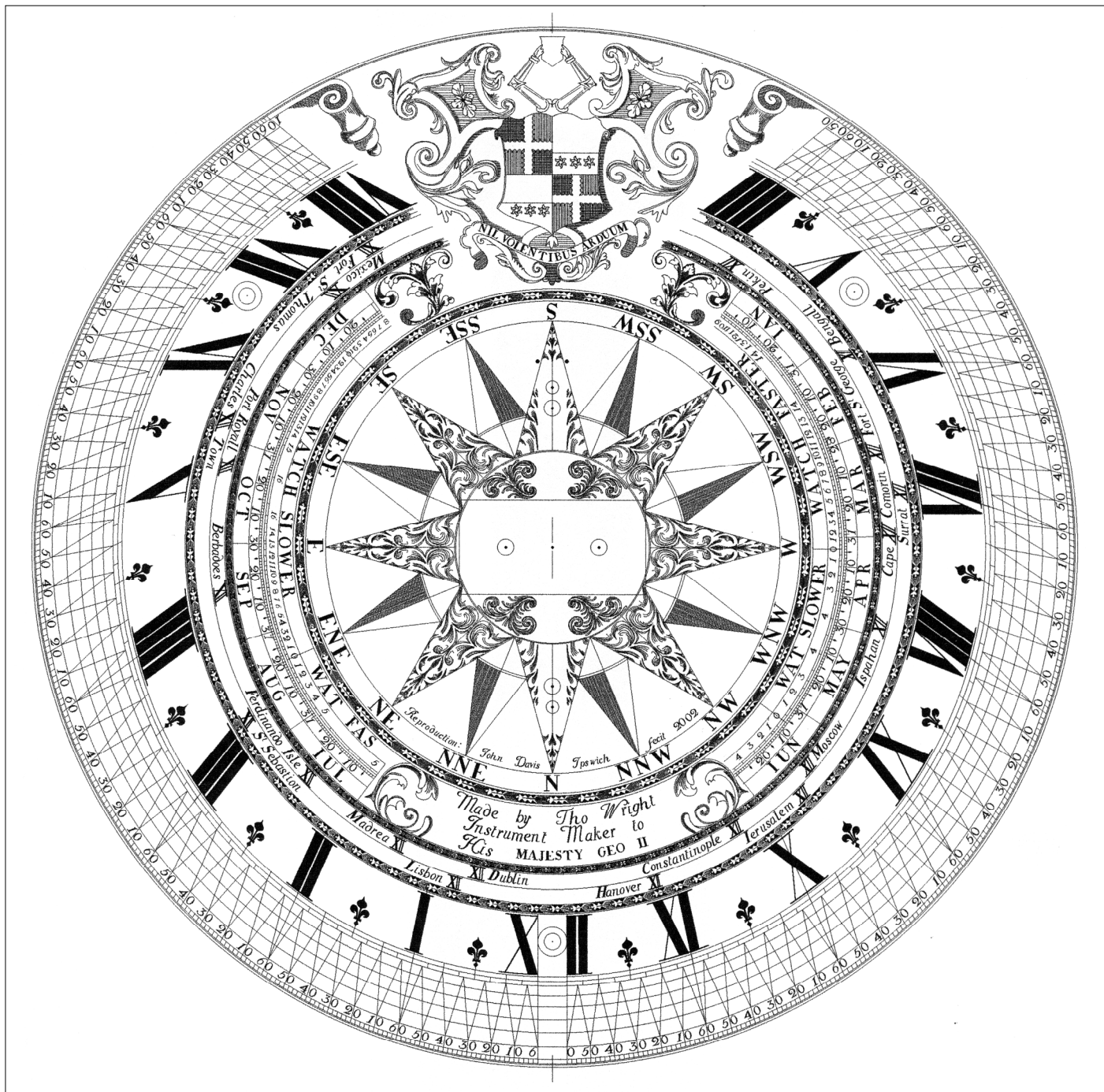
Fig. 3. A drawing of Wright's 18" dial for the Rudge family, as used for making the modern replica shown in Fig. 4.
