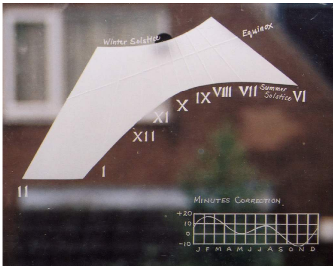
Fig. 3. Central portion of the engraved glass dial, with EoT/longitude correction graph.
