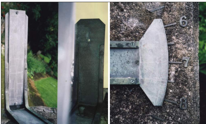
Figs. 6a, b. Details of the 1939 heliochronometer showing: a) left, the two sighting arms of the alidade and b) right, the time scale vernier on its end.
